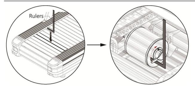
Pull up the rod of magnetic brake behind the motor with a tool (as rulers) to loosen the magnetic brake.
