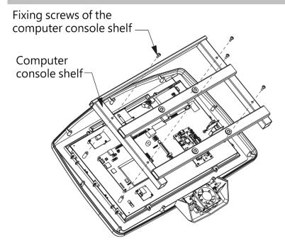
When change the panel, please make notice for the installation position of the wires, please do not plug into the wrong position. It is suggested to take a picture before changing. If the screen and other parts need to be changed, please loosen the fixing screws of the computer console shelf firstly, and then take off the shelf to change other relevant parts. After changing, test before use.
