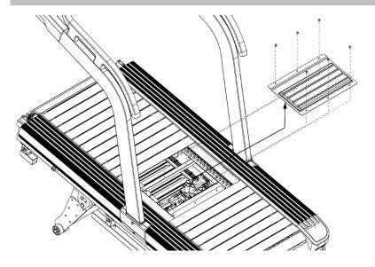
Abiding by the image to loosen the screw and take off the water-proof board.
