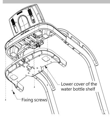
Take off the fixing screws, and then take out the lower cover of the water bottle shelf.
