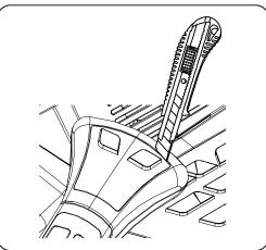
Embed the knife into the space between the control box and handrail to turn up the gel key to change the control box and gel key.
