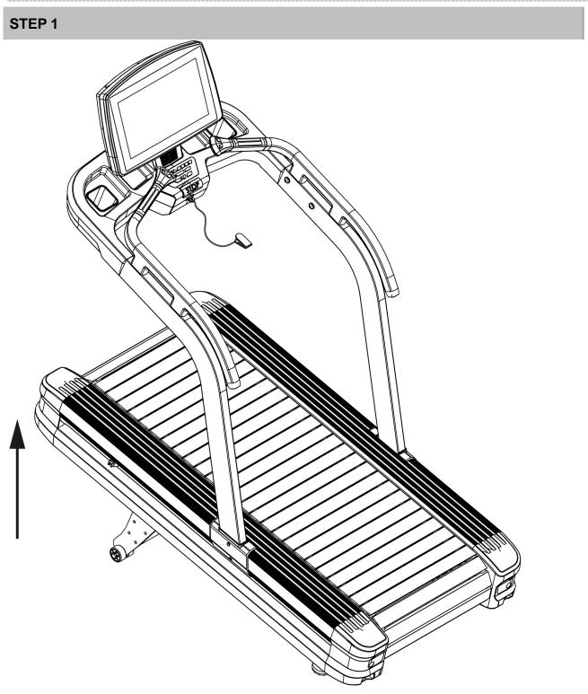
Firstly, incline the machine to the highest point, and then power off and plug out the power cable to keep the machine in this position.
