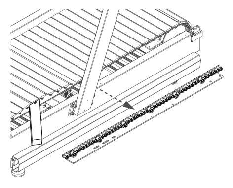
This step needs two person, one to heighten the running belt, the other to take off the front roller.
