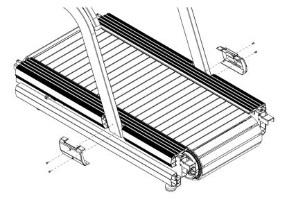
Pull up the decoration plate of the pedal lightly with screw driver to take off the pedal decoration plate.
