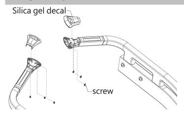
According to the image, take off the fixing screws, and then disassemble the air connector of the silica gel connection wire, tear up the old one and stick the new one to the rubber, and then connect the wire, finally lock back the screw.
