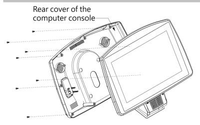
Loosen the fixing screws of the computer console, carry up the rear cover of the computer console and then take up the rear cover of the computer console.
