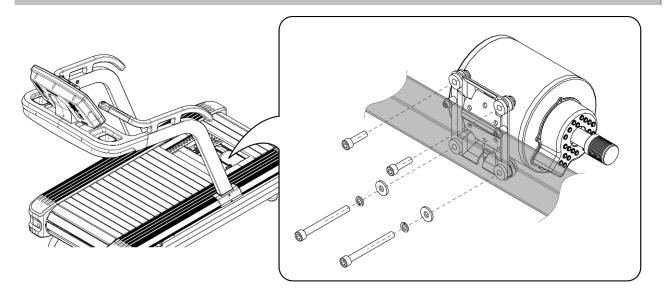
Turn the running board to the motor and loosen 4 fixing screws. Carry on the motor to take out the motor.
