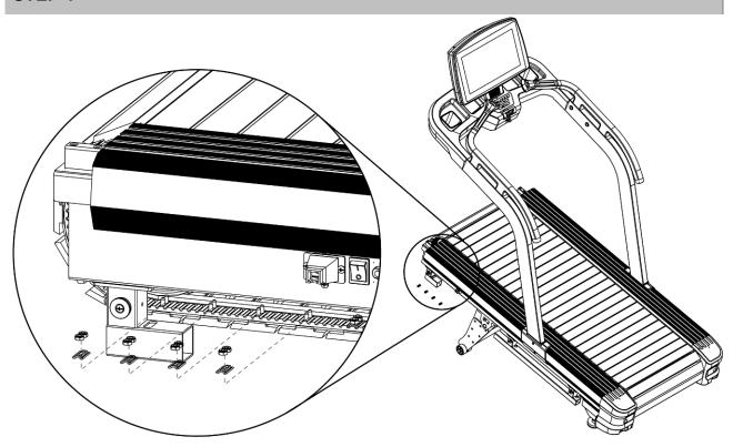
Loosen 4-5 pieces of nylon nuts and padding plated in the running board, according to the image.
