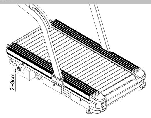
At that moment, please prepare two solid stuff to support at two sides of the frame to make the rolling wheel of the incline seat above the floor 2~3cm.
