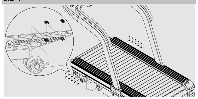
Loosen 4-5 pieces of nylon nuts and padding plated in the running board, according to the image.
