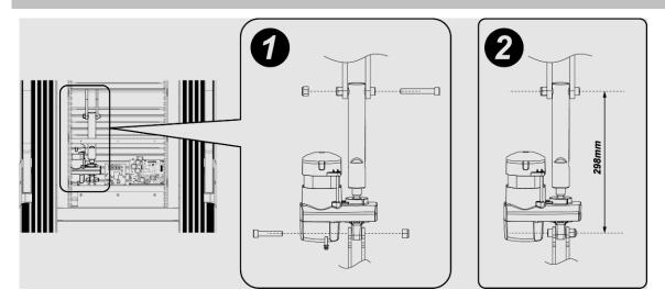
Firstly, plug out the wires, and then take off the screw and nylon nut in the bushings, finally, take off the screw and nylon nut in the frame to change the incline motor as the image 1.
