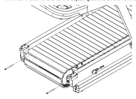
With hex wrench to take off the adjusting screws on the rear roller.
