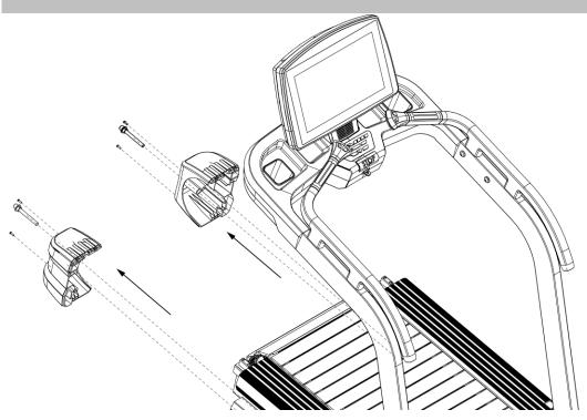
Loosen the fixing screws for the left and ring front adjusting caps, and take off the adjusting caps.
