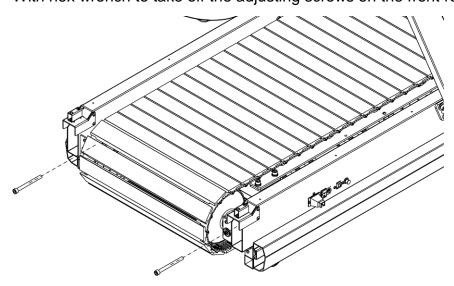
With hex wrench to take off the adjusting screws on the rear roller.
