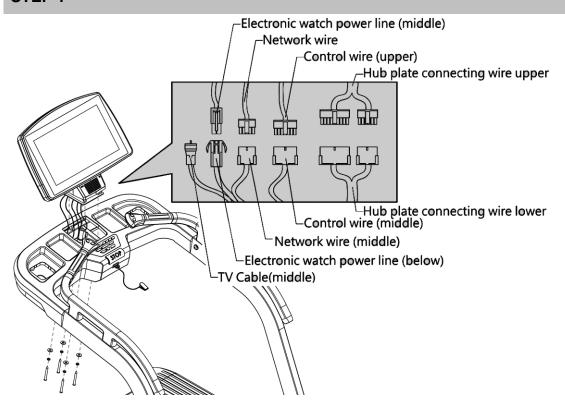
Take off the screw and washer in the computer console and water bottle shelf, and then plug out the wire to take off the computer console.
