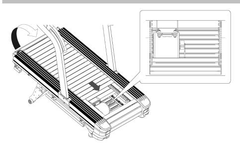
Turn the running board to the position where the motor can be seen clearly
