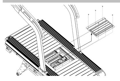
Abiding by the image to loosen the screw and take off the water-proof board.
