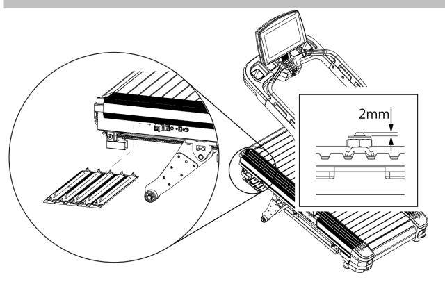
Take off the old running board and then assemble the new one.
