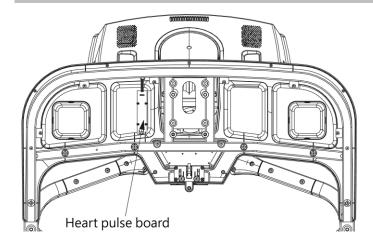
Pull out the wires of the wire collection board or heart pulse board, loosen the fixing screws to change new panel, after that, plug back the wires to the original positions. Finally, lock back the screws.
