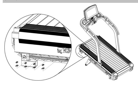
Loosen nylon nuts and padding plated at the left and right sides in the running board which should be changed, according to the image.
