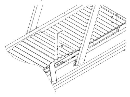
Take off the screws in the middle of the rail with cross screw driver.
