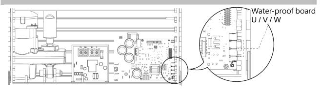
Pull out the motor wires (U.V.W)
