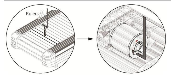
Pull up the rod of magnetic brake behind the motor with a tool (as rulers) to loosen the magnetic brake.
